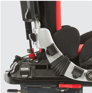
Back recline The point for rotation is close to the axis of the anatomical pivot point of the hip joints. This means that the back support maintains the correct position and minimises shear between the user and the backrest.
