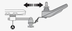
This is how you adjust the resistance of the rotational panel holder. Loosen or tighten the knob () on the friction joint to adjust how easily the rotational panel holder can be pushed to either side.
