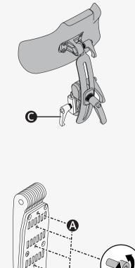
This is how you adjust the height and depth of the headrest.  $\checkmark$  Allen key 5 mm
