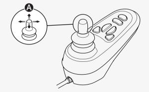
Do not move the joystick before, during, or immediately after you turn on the control system. If you move the joystick during this time, it can generate a joystick error. If this happens, turn off and then on the wheelchair.
