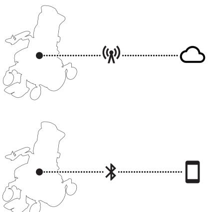
Your power wheelchair has a Power Platform, which contains a radio transmitter. In certain areas, radio transmission is not allowed and your wheelchair must be set to flight mode  $\bigstar$ .
