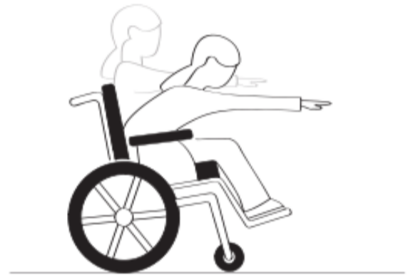
Figure 5.10: Forward reach in wheelchair
