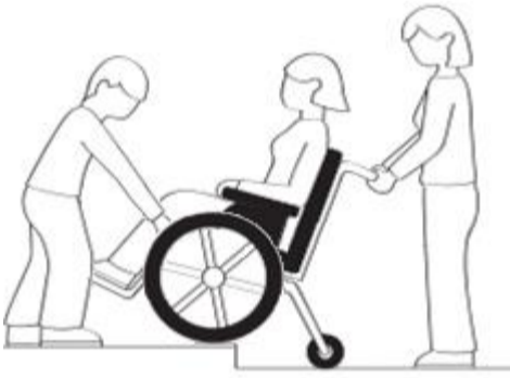
Figure 5.4: Assistant positioning for climbing curbs or single steps- method 2 in the Bentley LT-R
